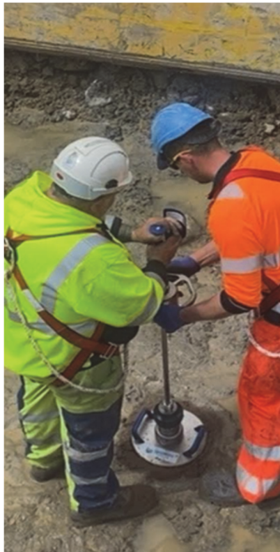
Figure 16 - FWD Test to Check Formation
