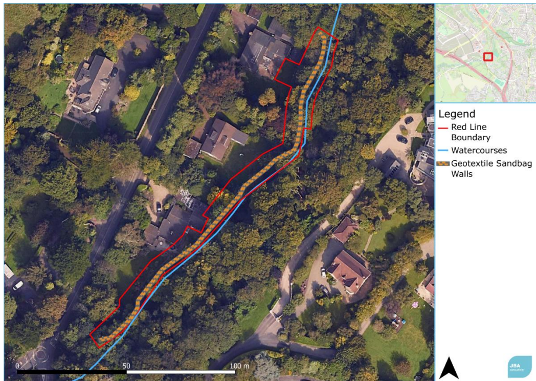
Figure 3-7: Indicative locations of sandbag walls (Cherrywood Road)
