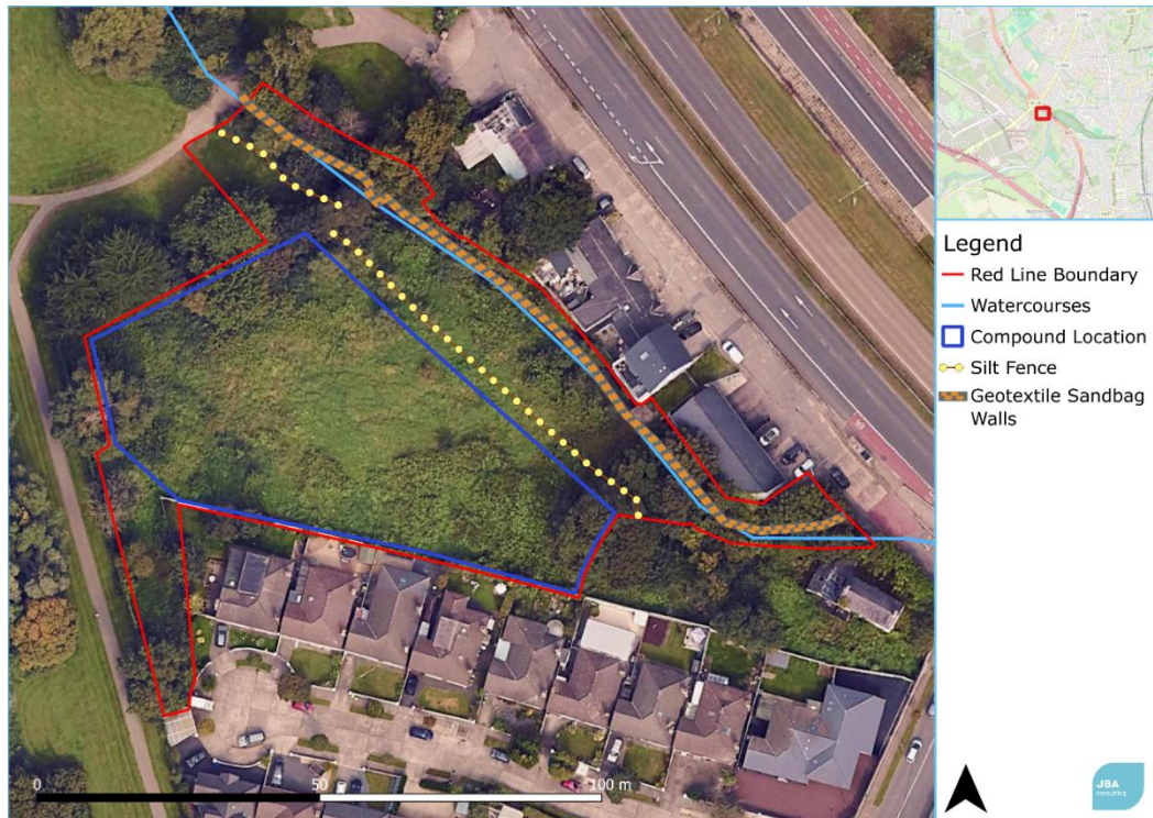
Figure 3-9: Indicative locations of silt fences and sandbag walls (Bray Road)
