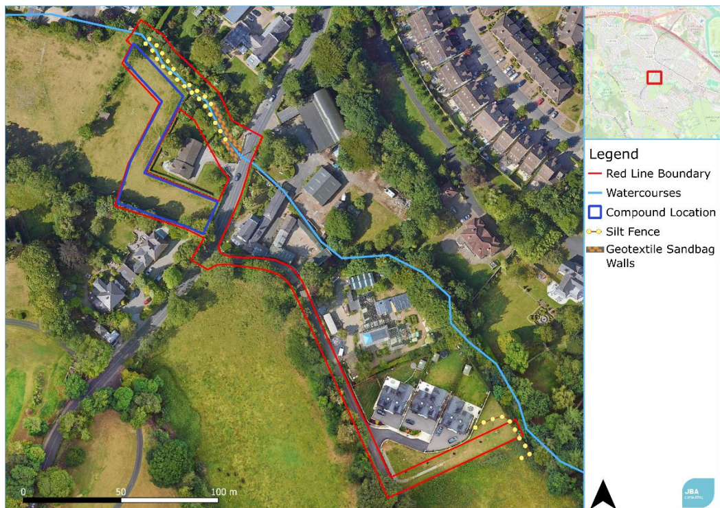
Figure 3-4: Indicative locations of silt fences and sandbag walls (Kilgobbin)
