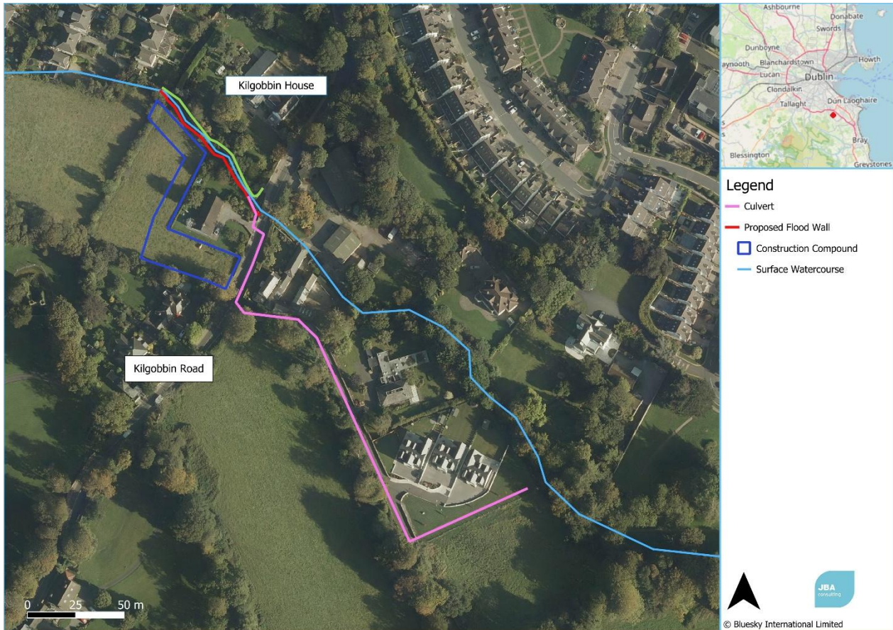
Figure 2-4: Kilgobbin Road Site Location
